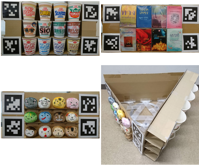
Figure 4: The three types of objects on the turntable as used in Experiment 1. The AR markers are used for the gaze tracker.
