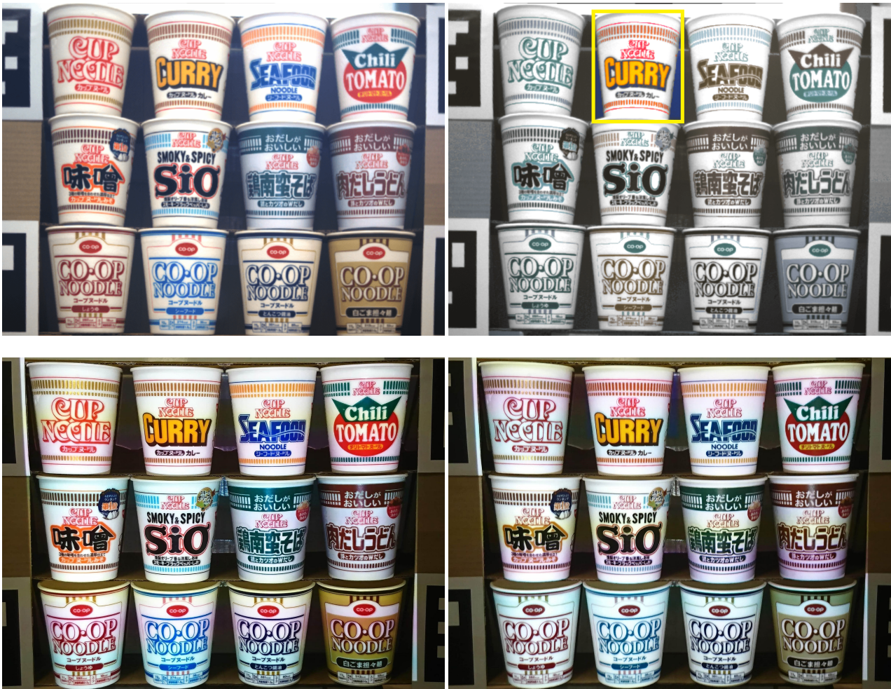
Figure 3: Examples of the shift and saturation filters. (a): an original image taken using a procam camera. (b): an image with the saturation filter applied, increasing the saturation of one object and inverting the colors of the other objects. (c): real objects on which the original image (a) is projected. (d): a real-world object on which the saturation-filtered image (b) is projected.
