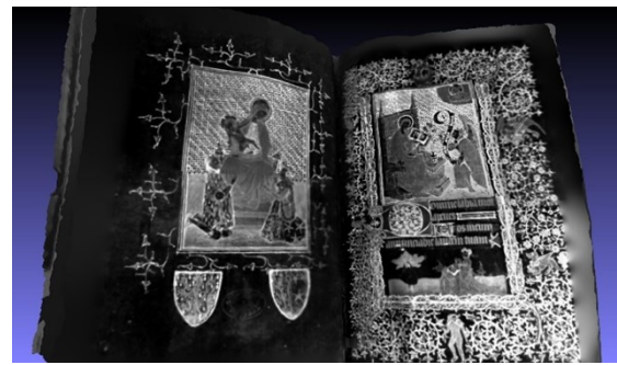
Figure 6: 3D mesh model of a manuscript obtained through SfM point cloud, using RGB images and IR thermal images as textures (Ms.459 Libro d'Ore, Angelica Library, Rome).
