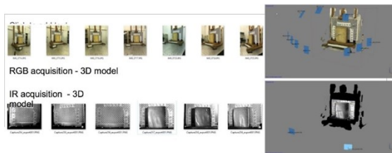
Figure 5: successful alignment test of RGB and IR images after lens calibration.
