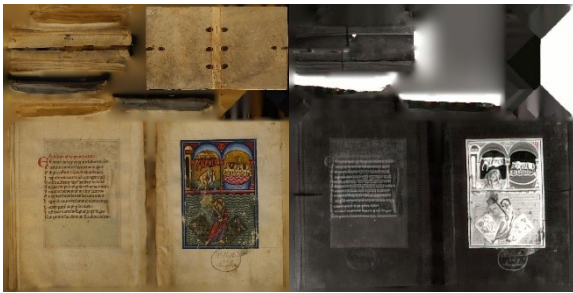
Figure 10: RGB and IR Atlas texture created in SfM software using texture building algorithms.
