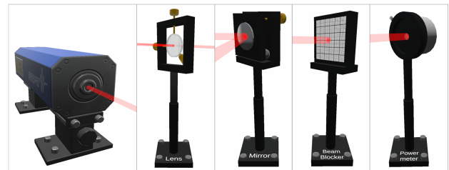
Figure 3: Examples of optical devices. From left to right: laser source, lens, mirror, beam blocker and power meter. In-game screenshots, retouched for visual clarity.
